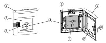
In the event of an alarm, the glass pane (2) is broken first, then the manual call point (3) is pressed hard. This activates the microswitch for alarm triggering and the indicator LED (4) blinks. A mechanism holds the pressed call point down.
