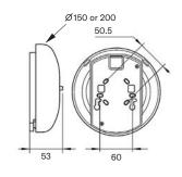
Mounting holes are provided to suit either BESA single gang installation boxes or for direct wall mounting
