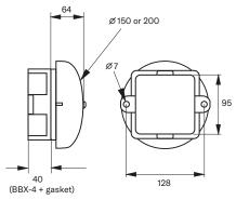
Mounting holes are located to suit BBX-4 installation box supplied.
